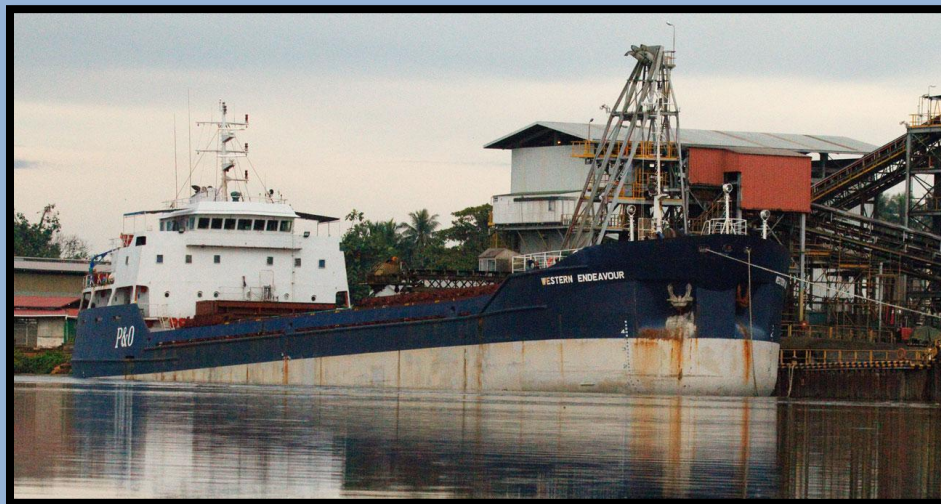
Western Endeavour – at Kiunga loading bulk concentrates. She was the first of the fleet of 6, 5000ton Mini-bulkers and 2 Tankers. The vessels were fitted with parabolic bows to assist in reducing wash, thus reducing erosion on the banks of the river.
